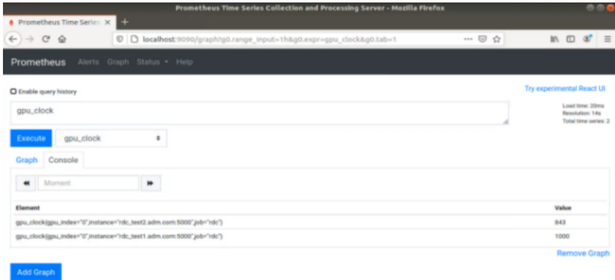
Fig. 5.1: The Prometheus image showing the GPU clock for both rdc_test1 and rdc_test2.
