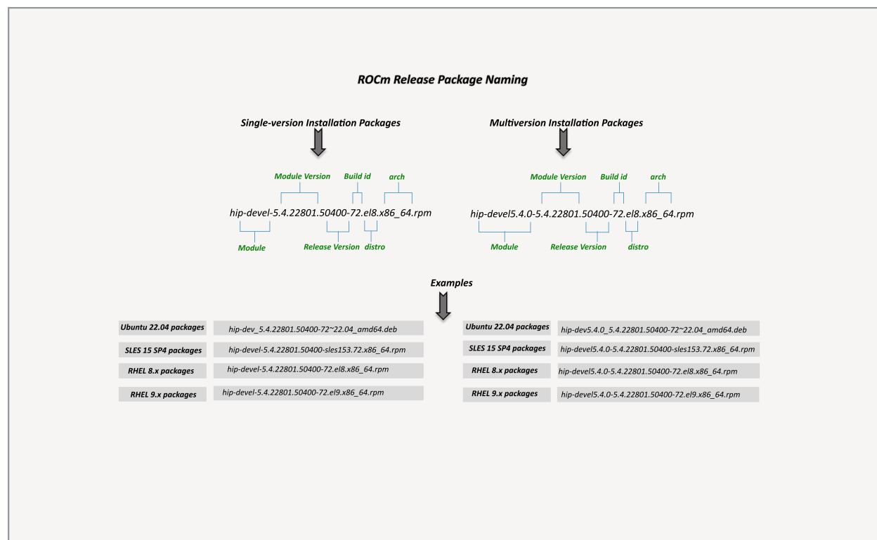
Fig. 3.2: ROCm Release Package Naming
